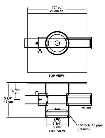
Pickup Tube Models: Single and dual tube pickup tubes available.
